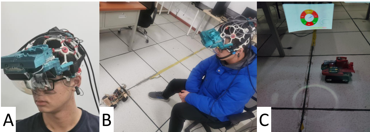
Figure 1: We present a system that combines an Augmented Reality device with Brain-Computer Interface technology, in order to make the training process of reading BCI for robotics control easier for the user. A) A user wearing a custom AR headset with built in EEG functions allows a wearer to control a robot. C) The first person view of the wearer. By using the headset to overlay the training software and controls on the target matter, we aim to allow faster training and control cycles with robotic platforms.
