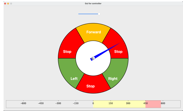
Figure 6: The Disk: A software solution that translates the visual output of the training, along with corresponding decisions to IoT actions. The disk system is displayed on the target for interactions via. the Ariel Supremacy.
